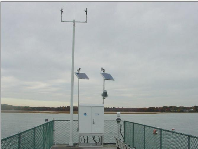
The Wells NERR also installed the first station of its kind that produces detailed tide, water level, and weather data that are sent via telemetry over a NOAA GOES satellite. This collaboration between Wells NERR and NOAA's Center for Operational Oceanographic Products and Services (CO-OPS) enables multiple data sets to automatically link.
